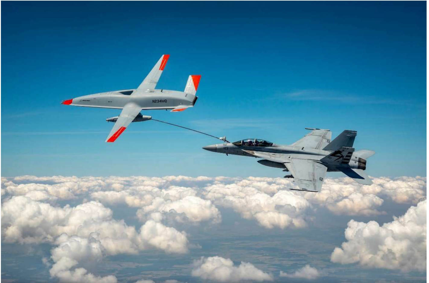
The Boeing MQ-25 Stingray (left) transfers fuel to a U.S. Navy F/A-18 Super Hornet on June 4, 2021, marking the first time in history that an uncrewed aircraft has refueled another aircraft. The MQ-25 was developed using Boeing’s advanced expertise in model-based digital engineering and design. (Boeing photo)
