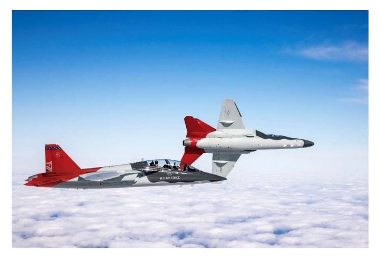
The Boeing T-7A Red Hawk has been recognized for its role in initiating the defense industry's digital revolution. The program used digital engineering processes, agile software development and an open architecture mission system to enable more rapid, affordable future aircraft development and affordable sustainment and is the model for all future defense programs. (Boeing photo)
