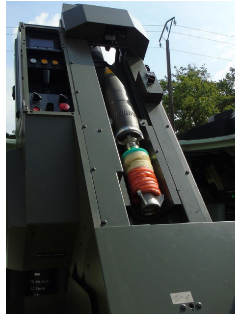
The 2R2M mounted in Renault Trucks Defense VAB 6x6 carrier. Image: Victor M.S. Barreira
