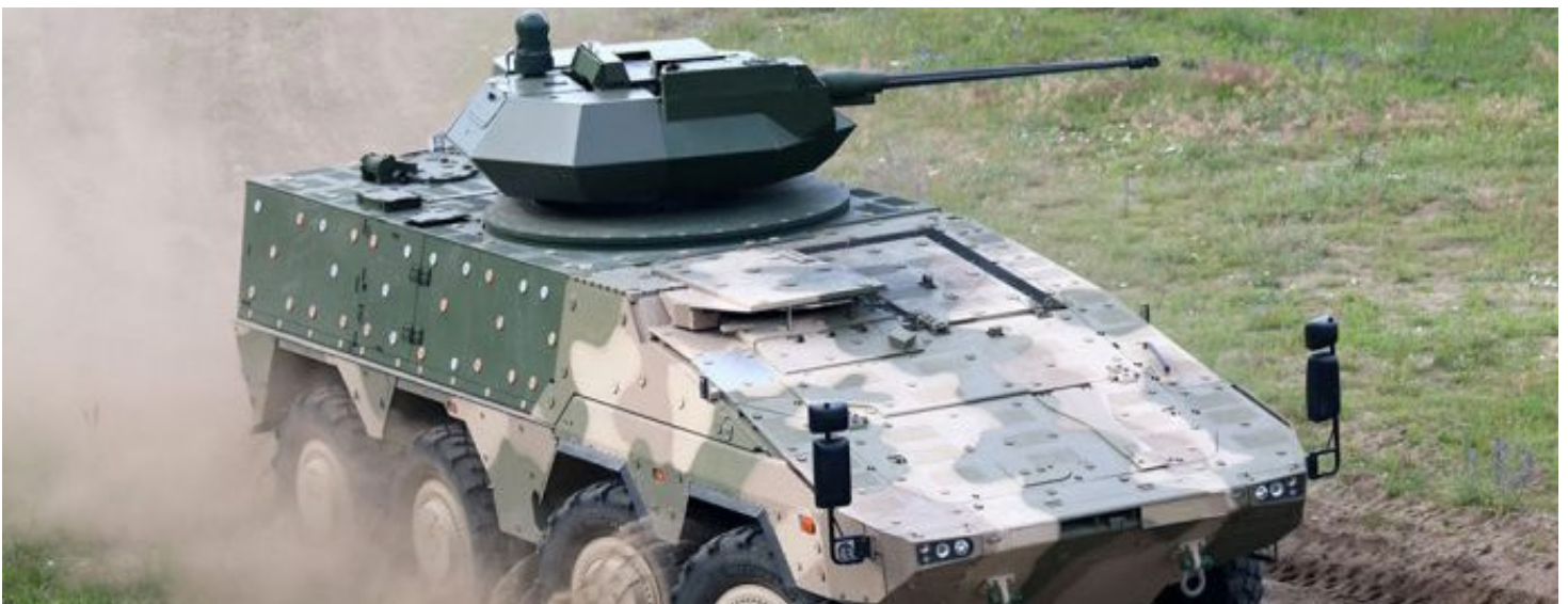
GTK Boxer 8x8 armoured with Samson Mk II remote weapon station. Image: Rheinmetall
