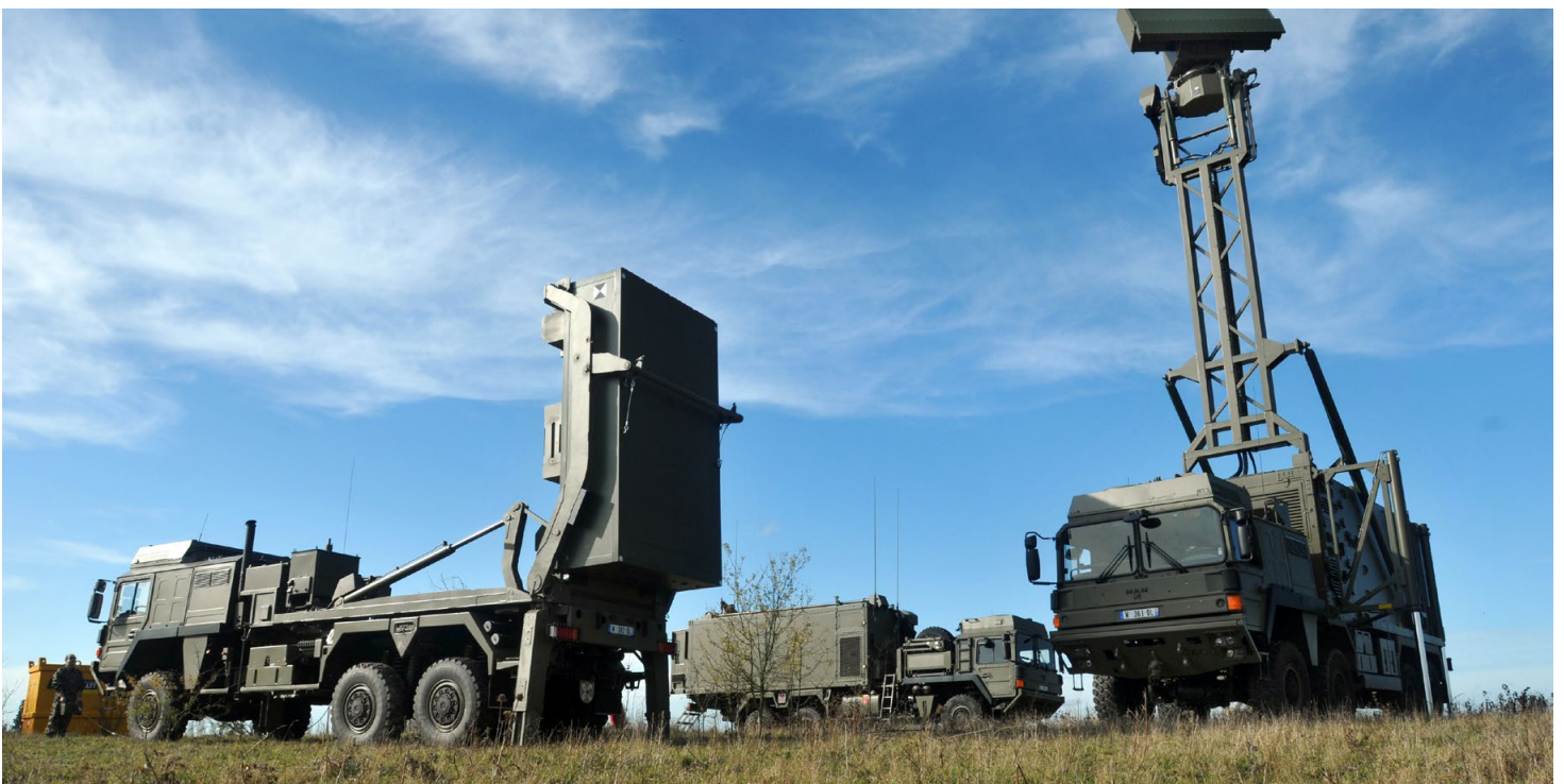
The VL MICA system here features launching, command and control and radar units (MBDA)
