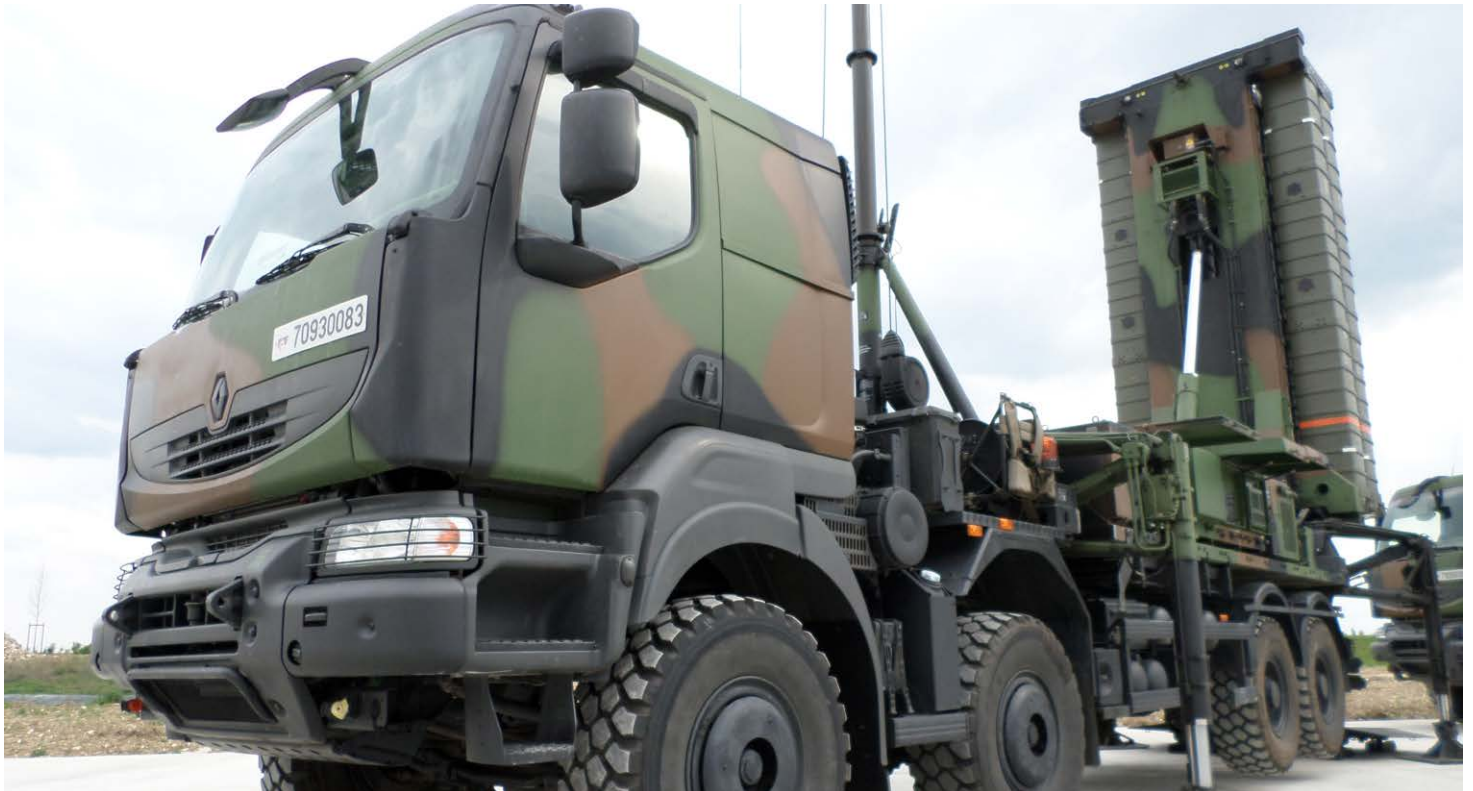
Each MLT launch platform is armed with up to eight missiles. Image: Victor M.S. Barreira
