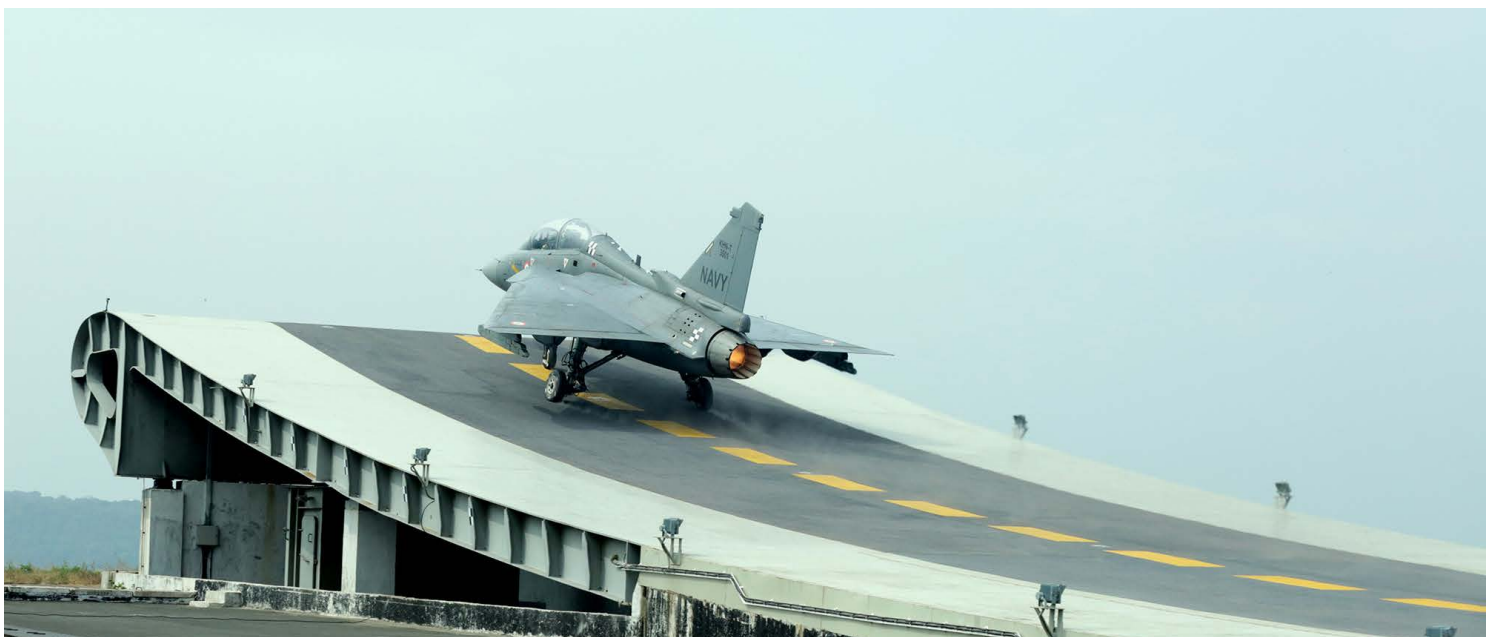
HAL Tejas NP-1 takes-off from the Shore Based Test Facility at INS Hansa, Goa. Image: Indian Navy
