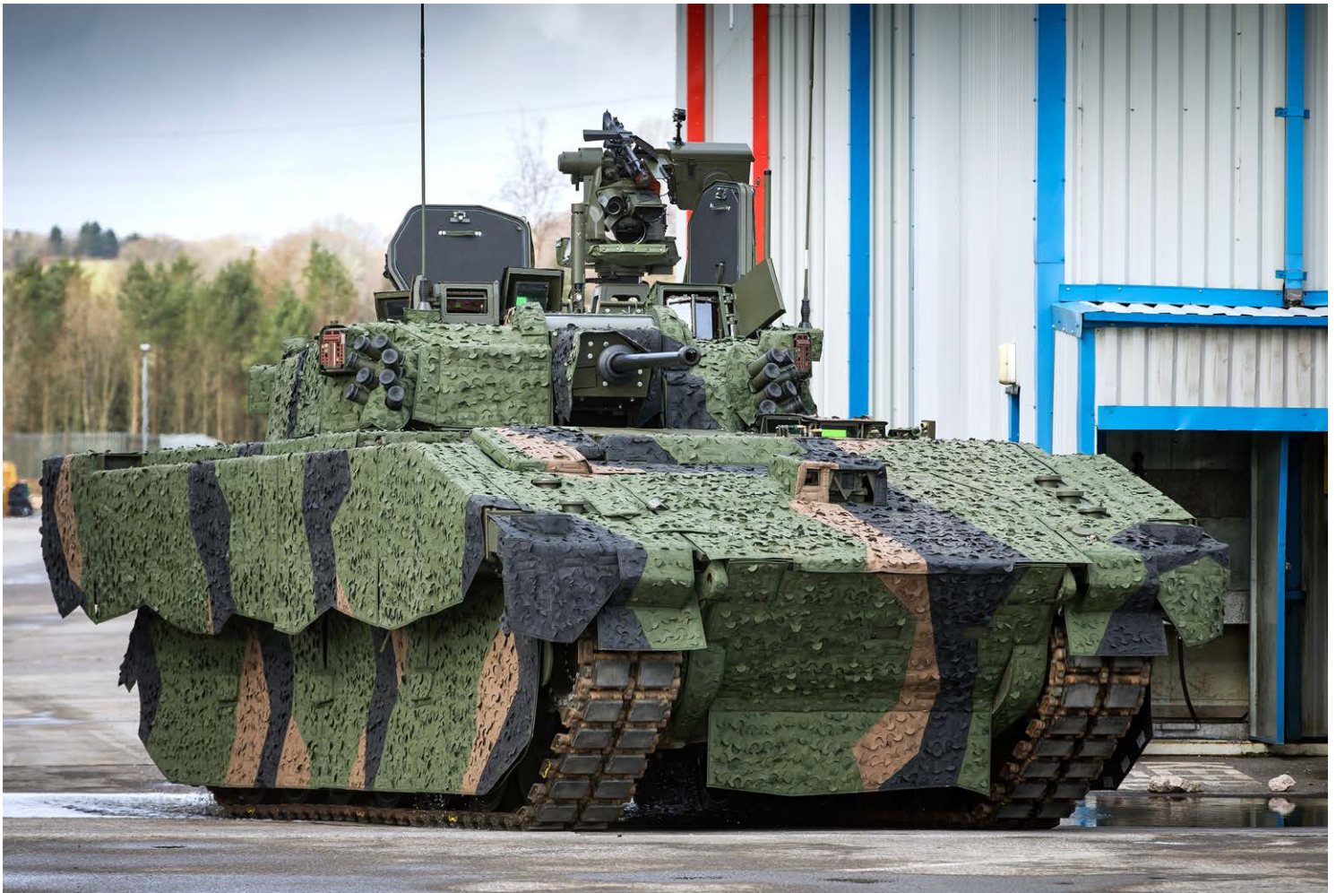
The Ajax armoured vehicle with CTAS turreted gun system. Image: General Dynamics UK
