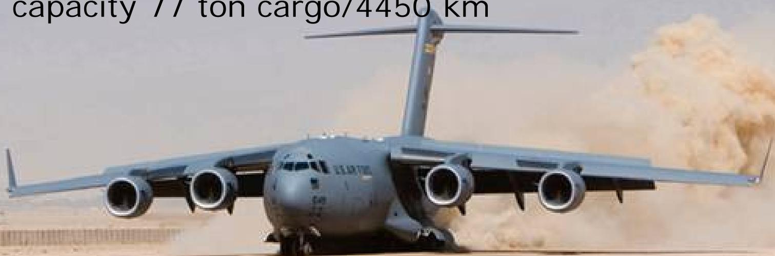
The C-17 is a large strategic transport aircraft capable of carrying 77 tons of cargo over 4450 kilometres and is able to operate in difficult environments and austere conditions.
